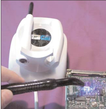
UV LED SpotCure-P provides lightweight, simple UV LED curing.
