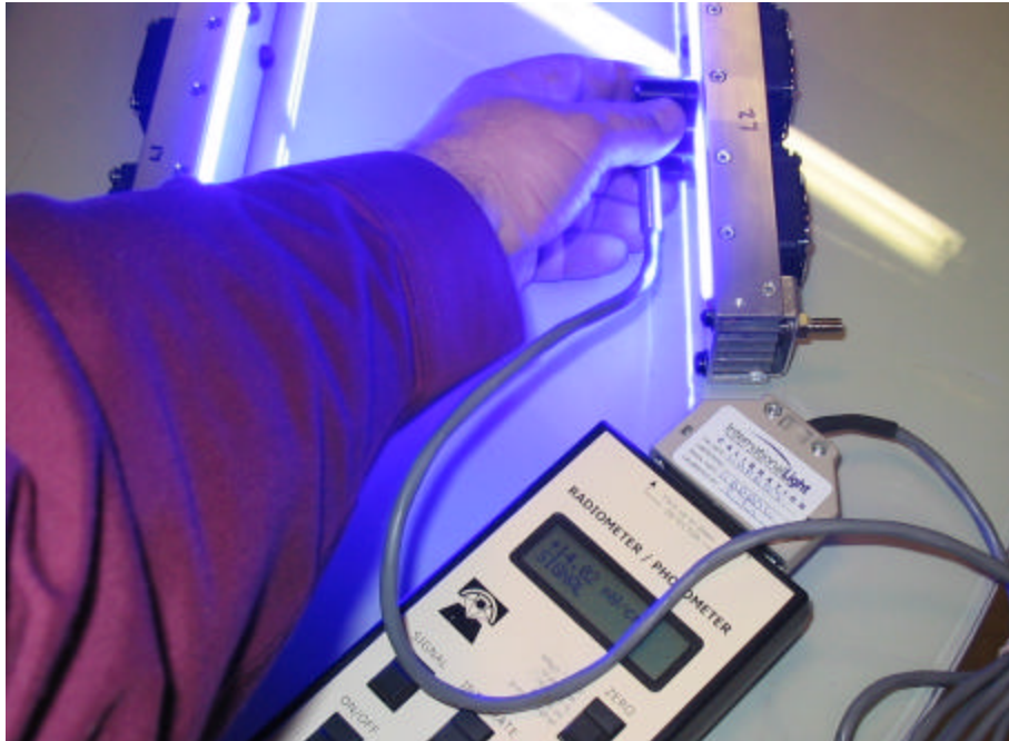
Figure 2 - Taking Light Power Reading
